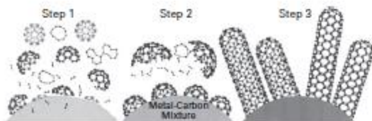
Fig 11: An illustration of a model for SWNT growth proposed by Kataura and colleagues [56].
